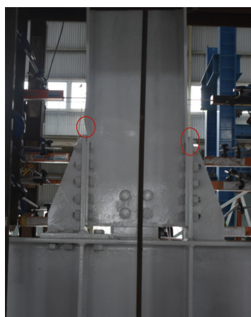
Figure 8. Cyclic Test Results Test Object 1
