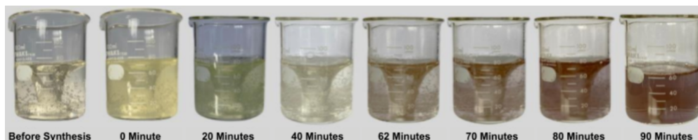
Figure 8. The Colour Change During the Synthesis Process of F1
