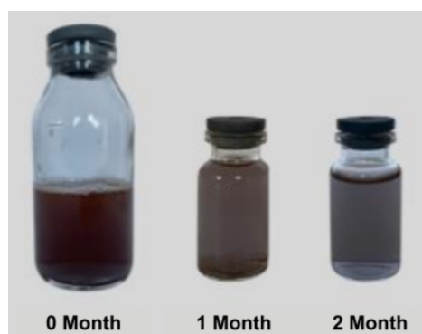
Figure 10. Colour Change Analysis of Gold Nanoparticles
