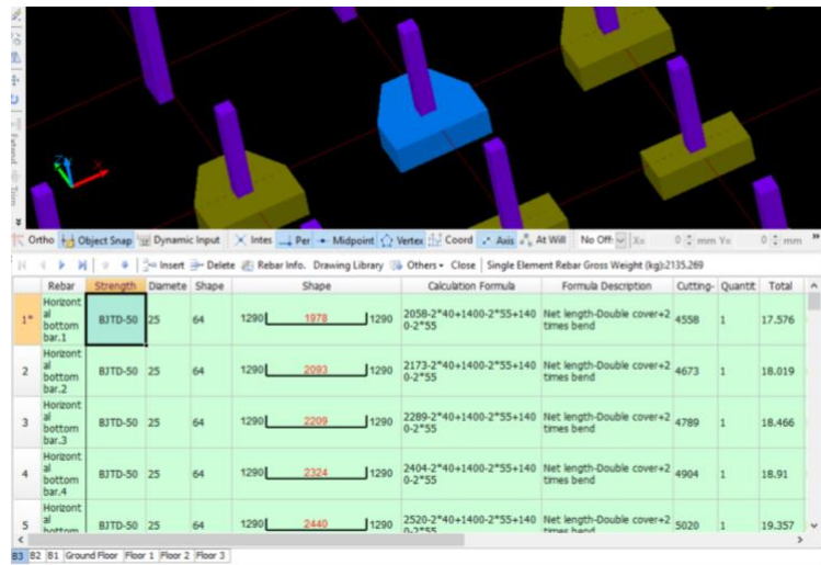
Figure 4. Rebar shape validation process
